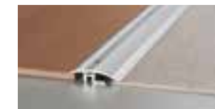
Adjustment profile PS400PEP Screwed, two-part aluminium profile for transitions between different height floor coverings
