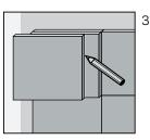
Do not apply too much pressure when placing the tiles in order to be able to remove them if necessary, because after the tile sticks, it is very difficult to remove.
